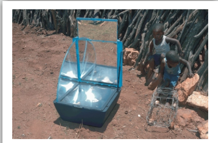
A solar box cooker with external reflectors
