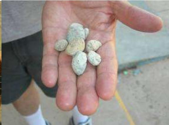
**Pumice used to insulate rocket stove.**
