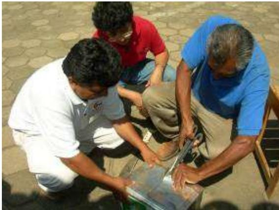
**Metal snips used to cut wind skirt.**
