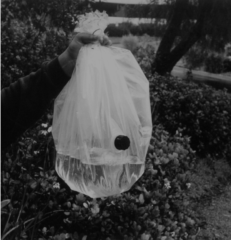
Fig. 6: The sack from a sack pasteurizer filled with water and tied shut.
